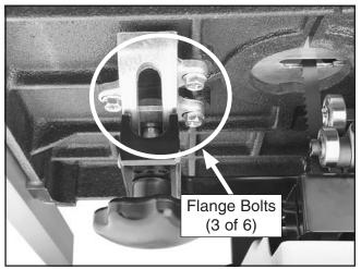
Figure 40. Location of trunnion bracket flange bolts.
